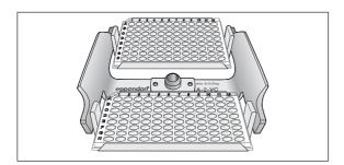
Insert the microplates and PCR plates (skirted) into the buckets.
